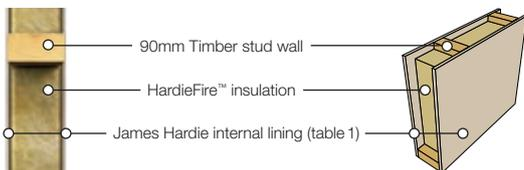
Designed for separating walls between sole occupancies in class 9c buildings; requiring a Fire Resistance Level (FRL) of up to 1 hour and an acoustic rating  $R_w \leq 45^{**}$ . This integrated solution will also provide you with excellent energy efficiency and bracing performance.
