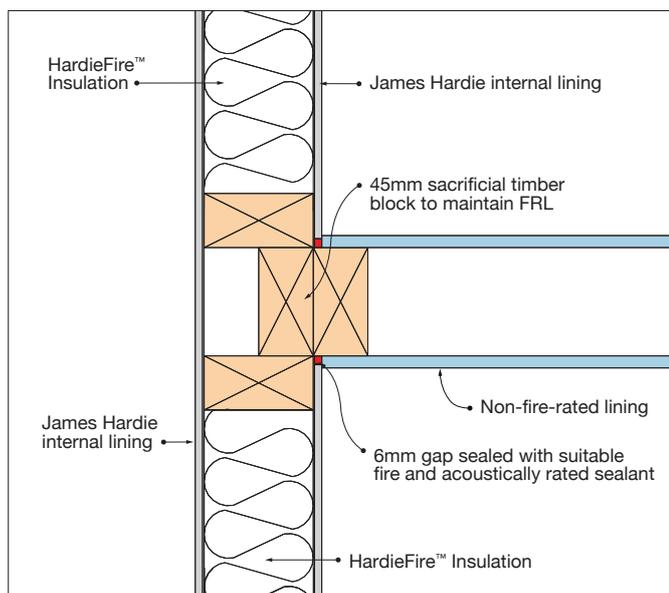
FIGURE 4 HARDIESMART™ AGED CARE WALL SYSTEM INTERSECTING NON-FIRE-RATED WALL
