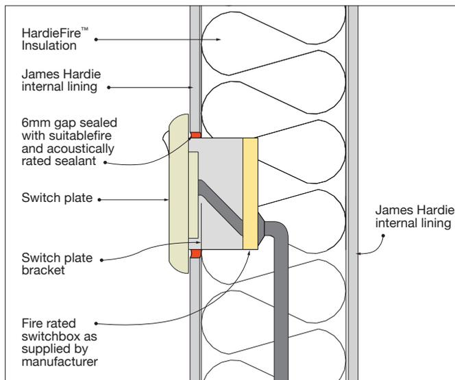
FIGURE 7 FIRE-RATED SWITCH PLATE OR GENERAL POWER OUTLET (GPO) ELEVATION
