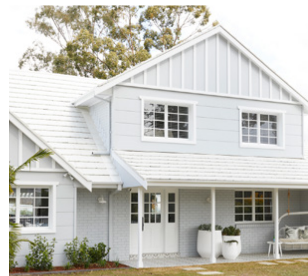
Hardie™ Flex Sheets Use with battens for cladding walls and gables.
